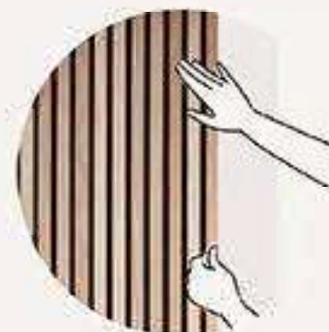
5. Put and press them to the wall
